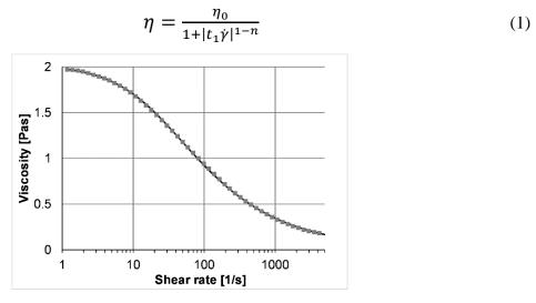
Figure 3. The viscosity of the polymer solution used (dots) and the fitted Cross-Williamson model (continuous line).
