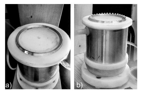
Figure 4. The spinneret mounted to a wooden stand, a) the sharp edges and the annular orifice, b) Taylor-cone formation at 0 rpm
